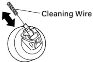
● Move the Cleaning Wire so that its tip comes out of the CO<sub>2</sub> Nozzle. The Cleaning Wire may touch the Cosmetic Nozzle depending on the angle. Do not press hard.
